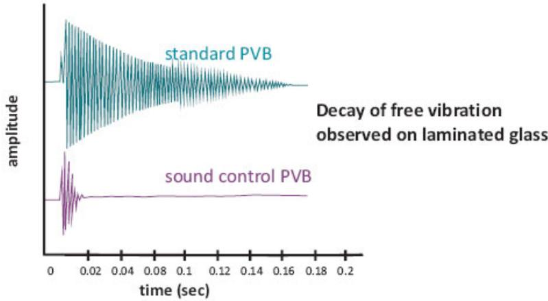
The sound-attenuation characteristics of PVB and acoustical PVB films can be understood by the following comparative graph. Considered here is the performance of a monolithic 4mm glass with a 4.76mm (2-0.76-2) regular PVB and 4.76mm (2-0.76- 2) acoustic PVB.
