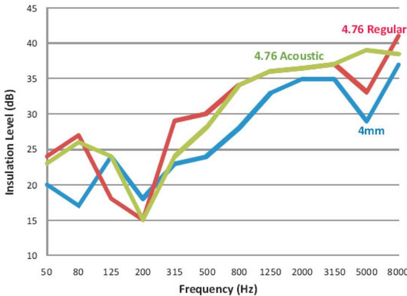
Although the transmission curve for 4mm monolithic glass is shifted to lower values owing to its slightly smaller mass if compared to the laminated glasses, the superior performance of the PVB glass (and more so in the acoustic PVB laminate) is clearly evident in the coincidence region. The reduced plate vibrations below 800 Hz also help enhance the sound-reduction properties of the laminated glass assembly.
