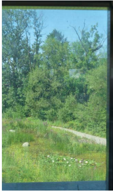
Illustration 6. Glass laminated with SEFAR fabrics. From inside the black fabric permits excellent visibility (left). Externally the fabric is metal coated. One of the effects is reduced reflectivity.
